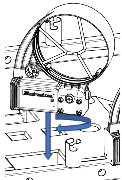
3. Place the beacons in the holder. By filling the pallet with the beacons, the beacon lights cannot be unlocked again. When unloading the pallet, the beacons must be removed first before the lights can be only then can the lights be unlocked and removed.
